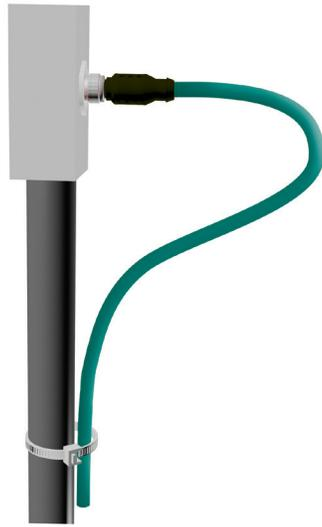
or shortening the cable's life span. The minimum bend radius is five times the cable diameter for stationary cables and 10 times for moving/flex cables. When cabling is bent beyond this pre-determined minimum bend radius, it can cause transmission failures. All pathways must maintain the minimum bend radius wherever the cable makes a bend.
